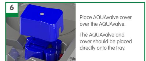
Place AQUAvalve cover over the AQUAvalve. The AQUAvalve and cover should be placed directly onto the tray.
