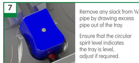
Remove any slack from ¼" pipe by drawing excess pipe out of the tray. Ensure that the circular spirit level indicates the tray is level, adjust if required.
