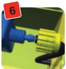
The AQUAvalve5 can now be connected to the 3/8" pipe. Unscrew the yellow collar and push the pipe through it. Push the 3/8" pipe onto the nozzle of the AQUAvalve5 and then replace the yellow collar by screwing it onto the AQUAvalve5.
