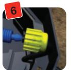
The AQUAvalve5 can now be connected to the 3/8" pipe. Unscrew the yellow collar and push the pipe through it. Push the 3/8" pipe on to the nozzle of the AQUAvalve5 and then replace the yellow collar by screwing it onto the AQUAvalve5.
